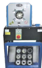
Uniflex crimping machine 扣压机(德国)
