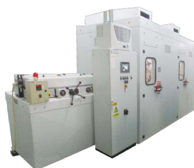
24锭德国进口 Mayer 编织机 (8台) 24锭意大利进口 OMA 编织机 (3台) Mayer 24-carriers braiding machine (8 sets) OMA 24-carriers braiding machine (3 sets)
