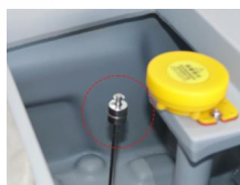
Large-opening recovery tank Water level sensor
