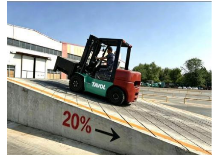
Forklift Gradeability Test
