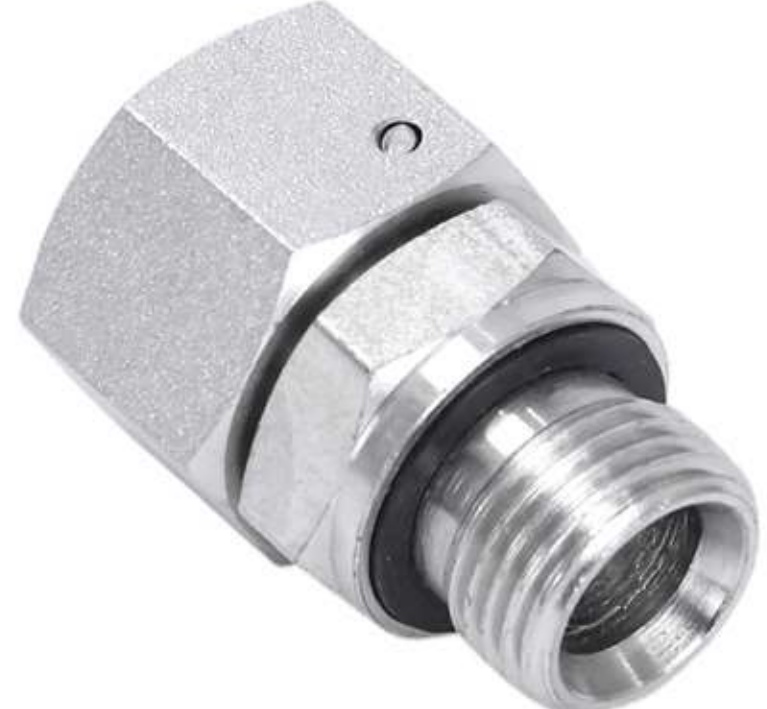
款号 NO. : 2BC-WD ITEM: BSP thread with captive seal / metric female 24° cone o-ring sealing 英管螺纹胶垫密封柱端/公制内螺纹24°锥带O型圈
