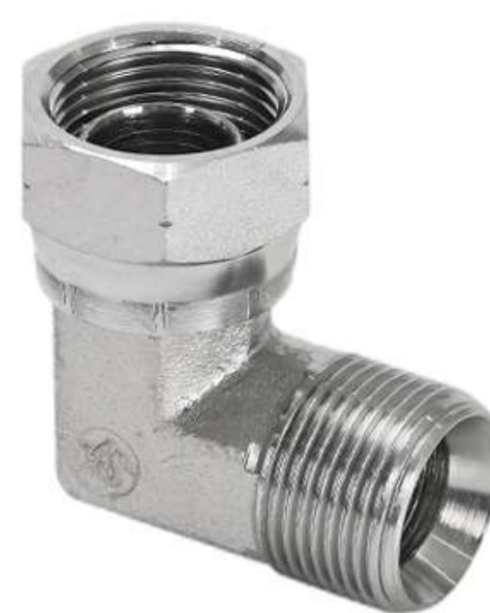
款号 NO. : 2B9 ITEM: 90° BSP male double use for 60° seat or bonded seal/BSP female 60° cone 90°弯英管外螺纹60°内锥/英管外螺纹60°内锥弯头
