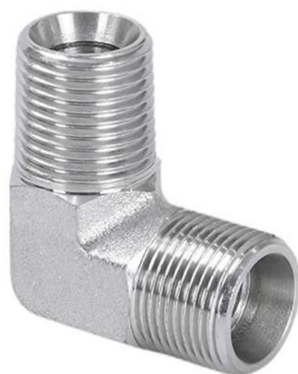
款号 NO. : 1CT9 ITEM: 90°BSPT male /metric male 24°cone l.t. 90°英椎管外螺纹弯头
