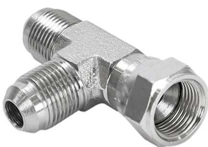
款号 NO. : CJ ITEM: JIC male 74°cone / JIC female 74°seat run tee 美制JIC外螺纹74°外锥/74°内锥主支三通
