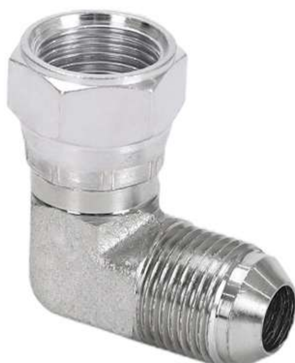
款号 NO. : 2J9 ITEM: 90°JIC female 74°cone / JIC male 74°cone 美制JIC外螺纹74°外锥/JIC内螺纹74°内锥 弯头
