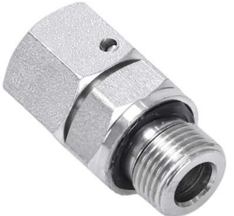
款号 NO. : 2GC ITEM: BSP thread stud ends with o-ring sealing / metric female 24° cone o-ring sealing 英管螺纹O行权密封柱端/公制内螺纹24°锥带O型圈
