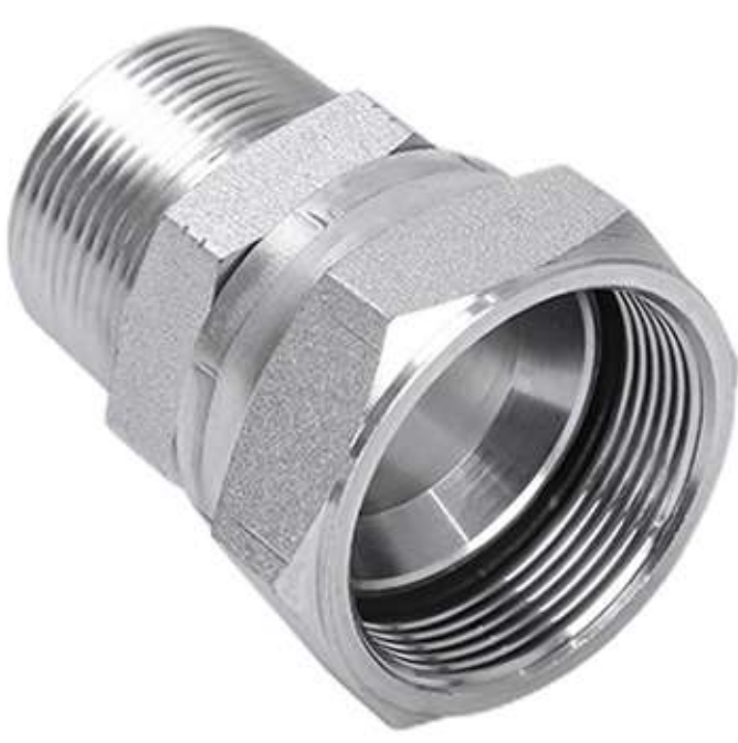
款号 NO. : 2NJ ITEM: NPT male / JIC female 74° seat NPT外螺纹/JIC内螺纹74°内锥接头
