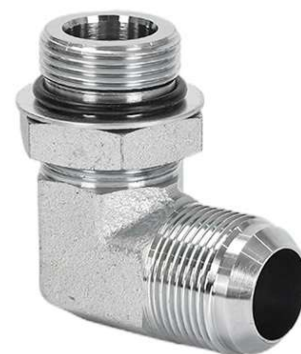
款号 NO. : 1J09 ITEM: 90°elbow JIC male 74°cone /sae o-ring 美制JIC外螺纹74°外锥/SAE外螺纹弯头带胶圈
