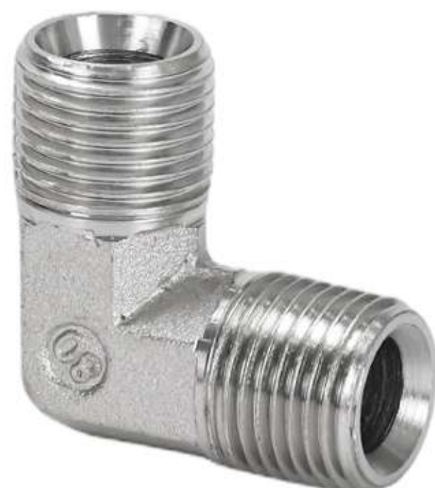
款号 NO. : 1BN9/1BT9 ITEM: 90° elbow BSP male 60° seat/NPT male 90°英管外螺纹60°内锥, 美制NPT外螺纹/英椎管外螺纹弯头
