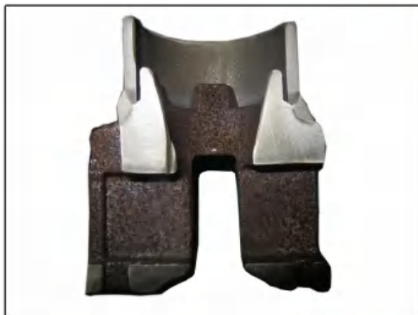
Casting end with tube welding
