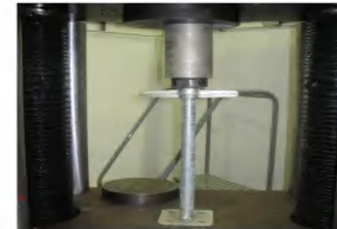
Base Jack (Test in different nut high)
