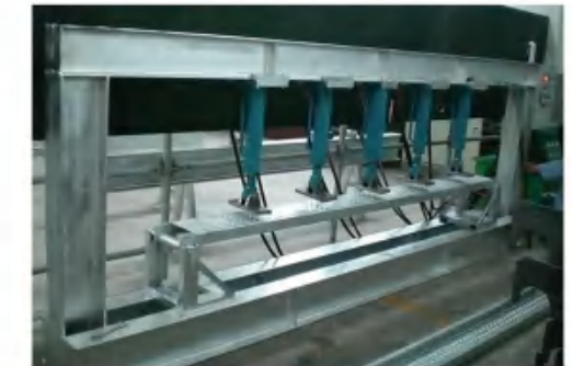
Steel Plank (Uniformly distributed load test)
