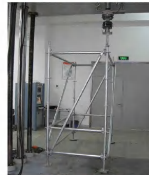
Ringlock Standard (Load capacity of single standard)
