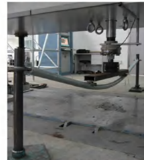
Ringlock Ledger (Load capacity test)
