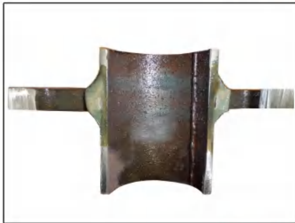
Rosette with tube welding
