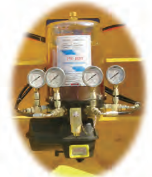
Centralized lubrication with shaft-end pressure monitoring
