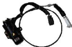
CAT305-307 throttle motor Applicable model:E305E/E307E
