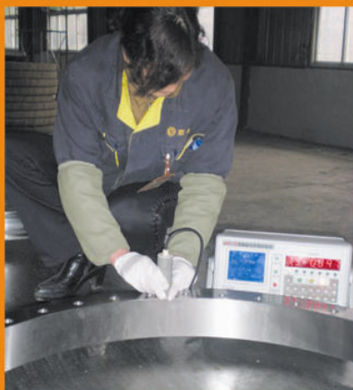
裂纹检测 Crackle Inspection
