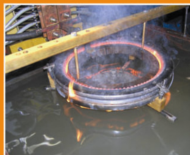
整体齿淬 The Whole Teeth Quenching
