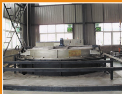
回火炉 Tempering Furnace
