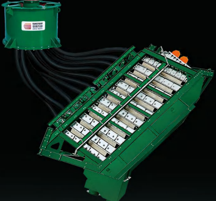
FY-HVS-10-1214 十层高频筛 FY-HVS-10-1214 Ten-deck High Frequency Screen
