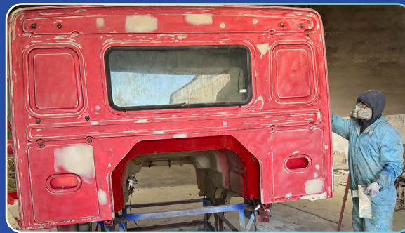
Preparation: Degreasing, leveling, and sanding
