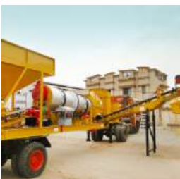
Mobile Drum Mix Plant
