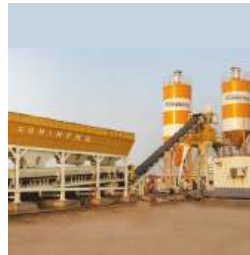
Concrete Batching Plant
