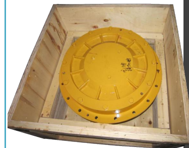
右振动室 VIBRATORY HOUSING-RH 22W0012
