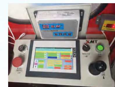
Control panel for operator's cabin 驾驶室用操作台
