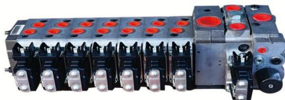
电液一体化压力流量控制系统 Electro-hydraulic integrated pressure and flow control system
