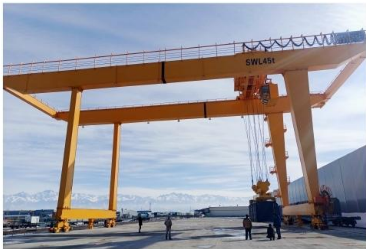
◆ RMG轨道式集装箱门式起重机 RMG rail container gantry crane
