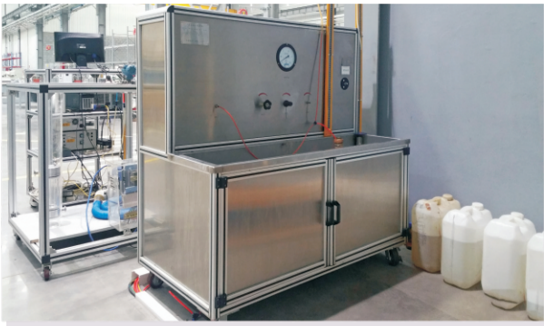
滤材冒泡点检测台 Bubble Point Test Machine
