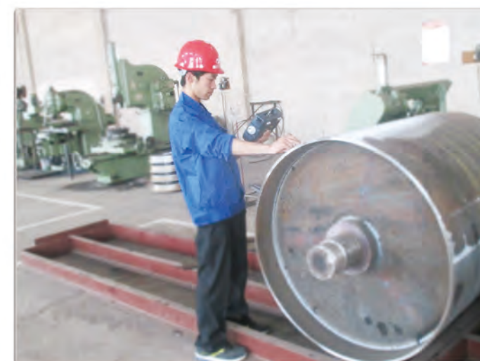
▲ Flaw detection inspection of pulley shaft 滚筒轴探伤检测
