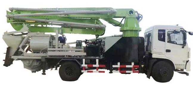
臂架泵 Boom pump truck
