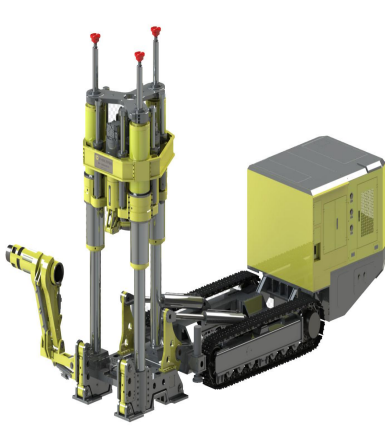
自行式天井钻机 Self-propelled courtyard drilling
