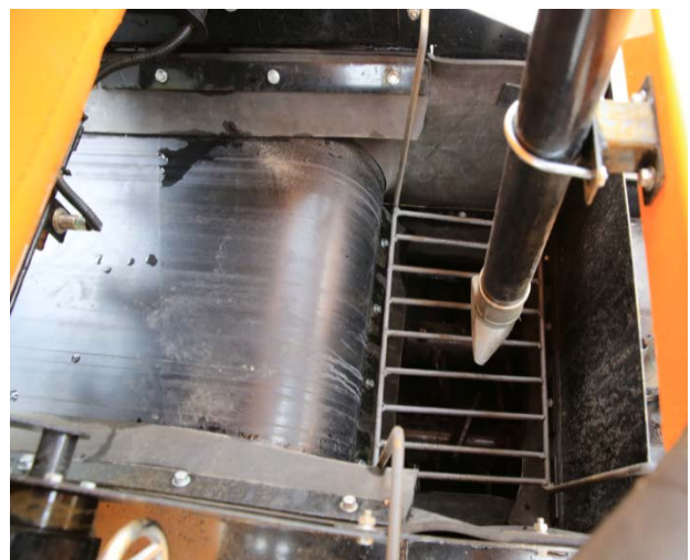
Stable belt feeding system
