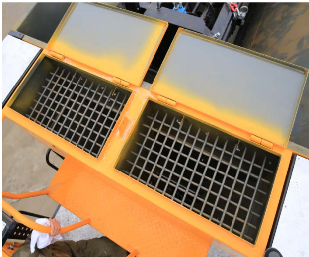
2 mineral fillers tank
