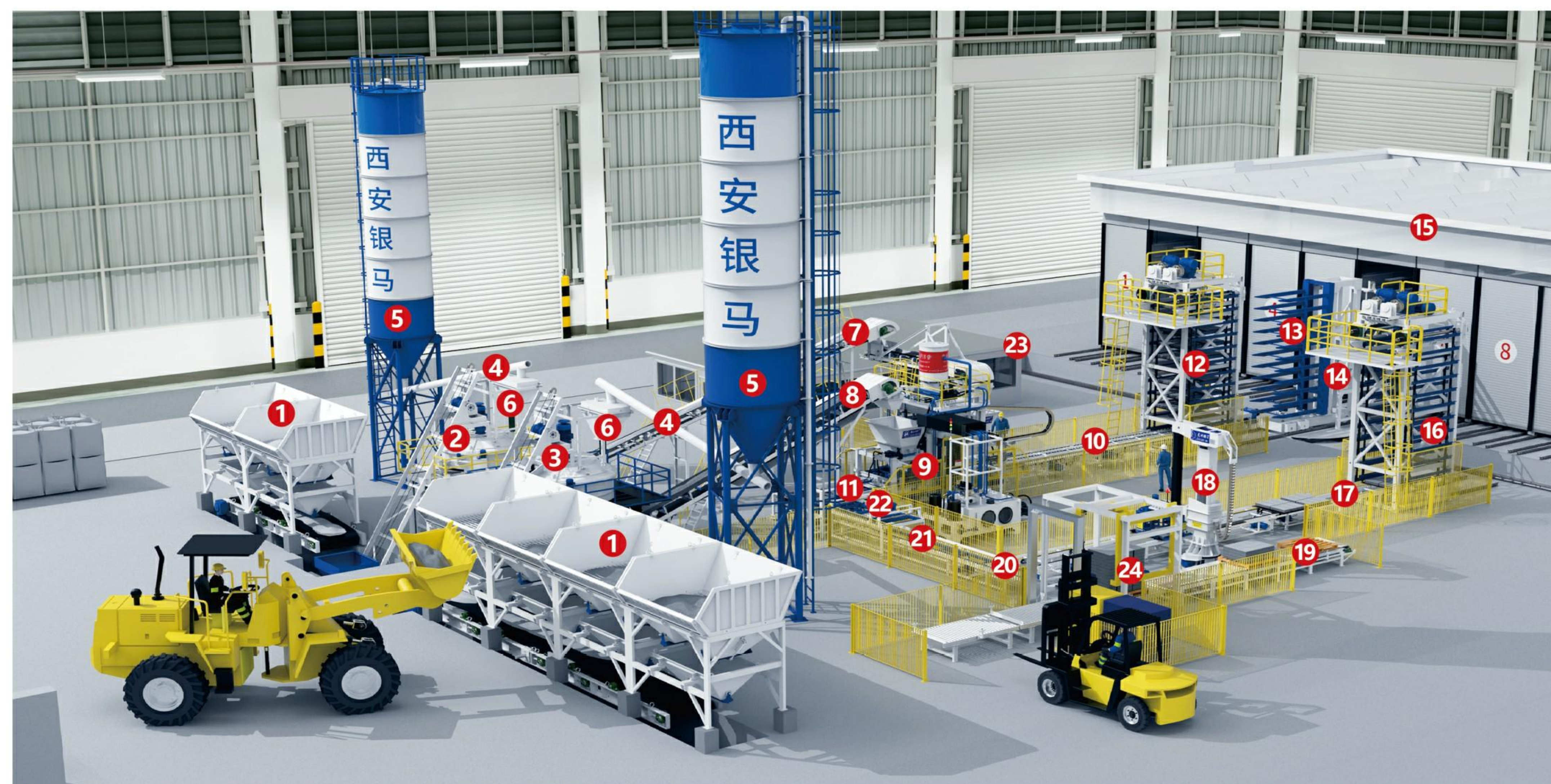
The arrangement of fully automatic block/stone making production line
