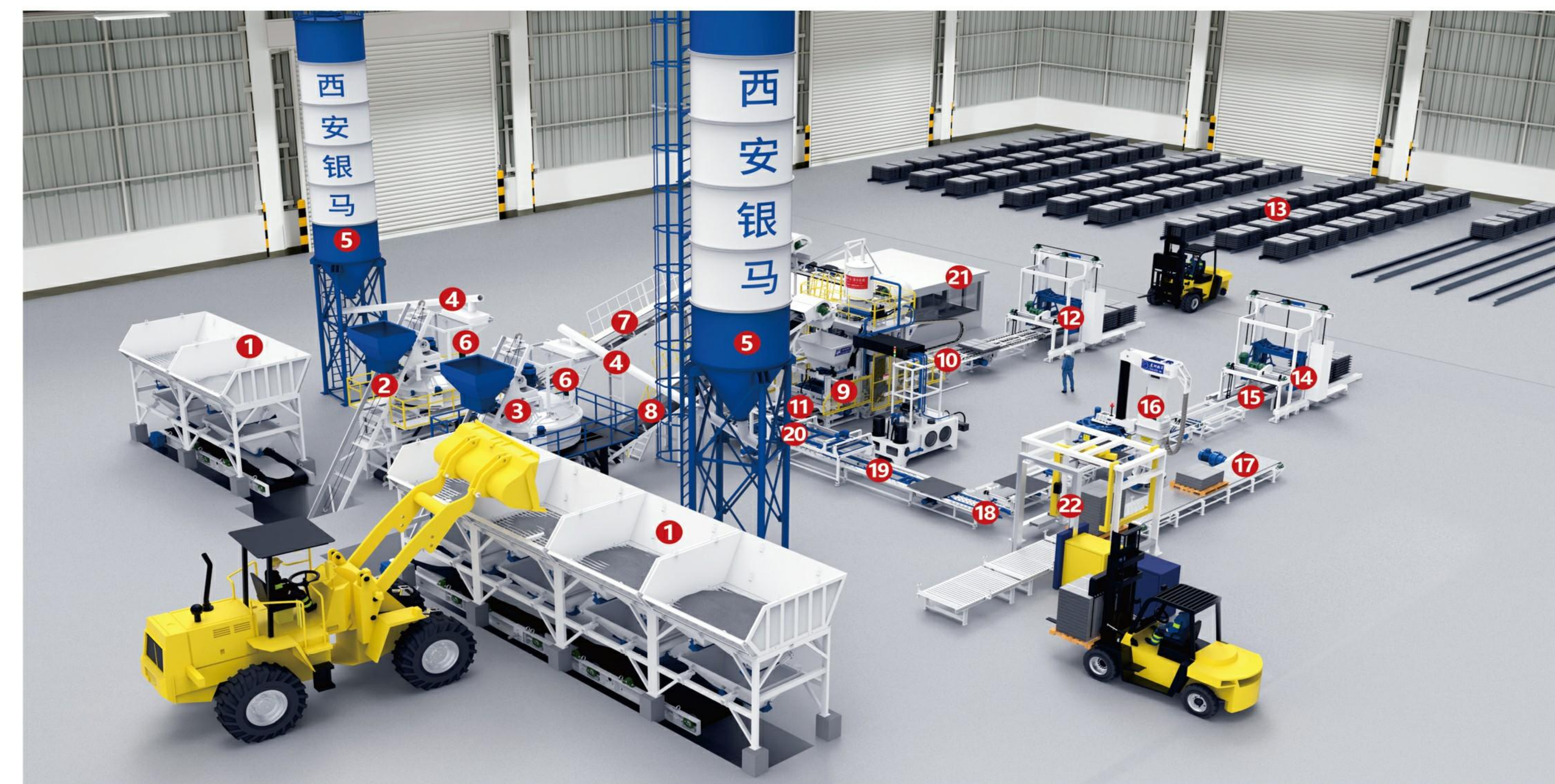
The arrangement of automatic block/stone making production line with open cycle
