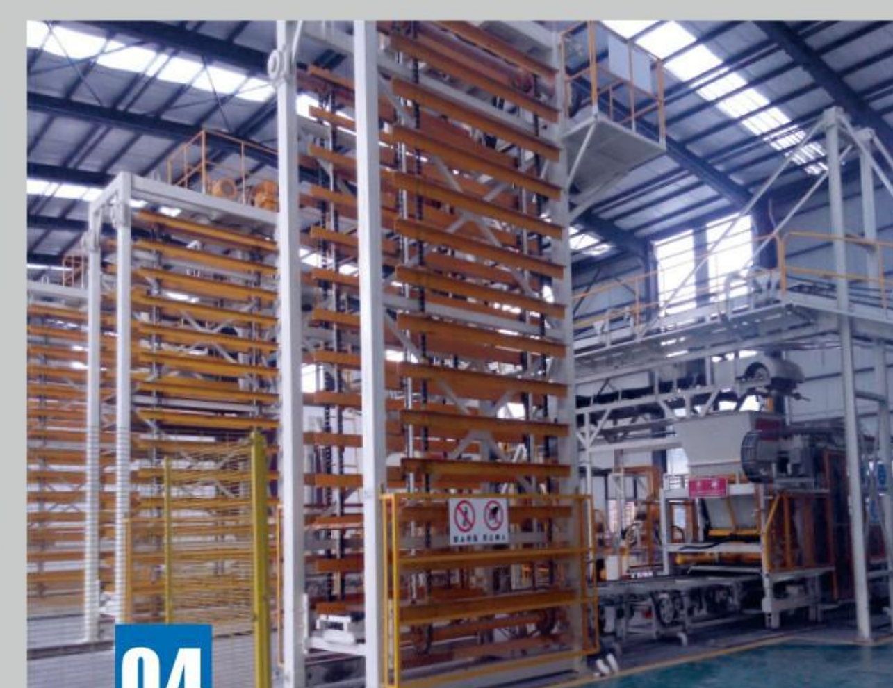
04 Ascending/Descending slab system
