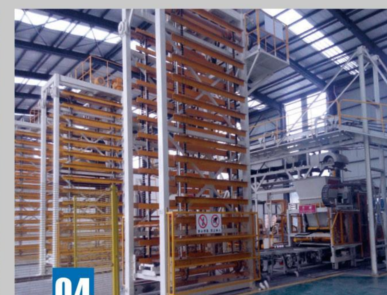
04 升降板系统 Ascending/Descending slab system
