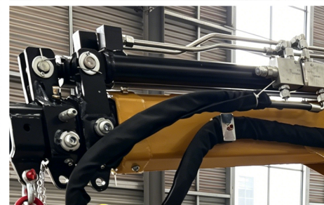
Hydraulic Cylinder & Hoses
