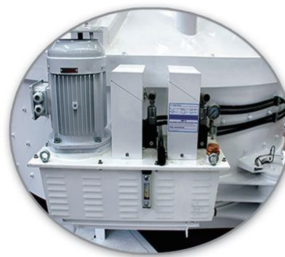
Offers both hydraulic and pneumatic discharge systems with configurable discharge gates (1-3 openings)
