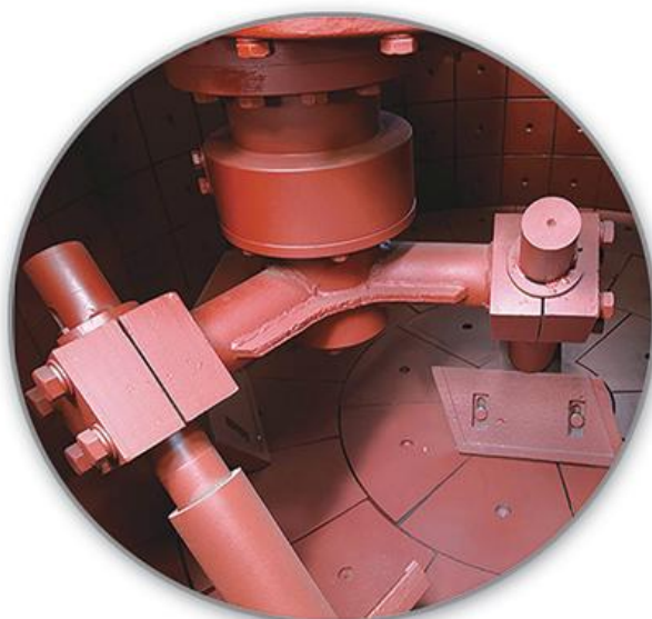
Mixing arms feature a modular block design with dedicated wear-resistant sleeves
