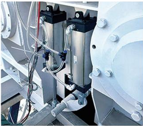
Dual-Cylinder Discharge System
