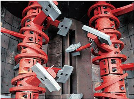
Anti-Build-Up Shaft Design
