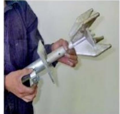
(3) 安装专用顶托等部件 Assemble the prop head and steel prop with spring bolt
