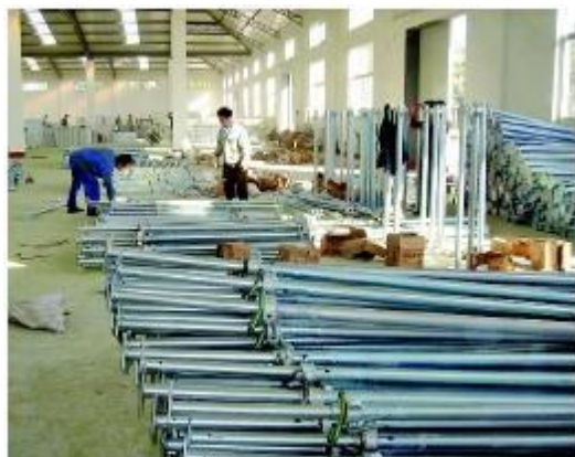
对钢支撑逐根的验收 Inspection for the steel props
