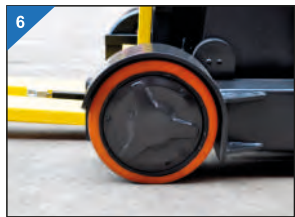
ASC forklift active stabilization system When the mast moves forward and backward, the service brake will be locked automatically, which can ensure truck does not move forward and backward, improve the stability of the truck.
