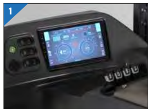
Fully upgraded console Large-screen instrument and finger-tip sticks, adopt Germany ELOBAU, with ergonomics design, can display battery power, wheel angle, faults and other information.
