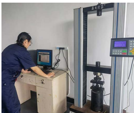
Bending Strength Inspection
