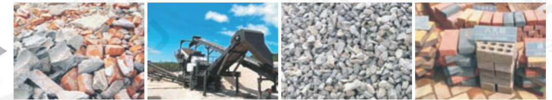
混凝土废料 concrete waste 破碎、筛分 crushing and screening 再生骨料 recycled aggregate 再生混凝土产品 recycled concrete products
