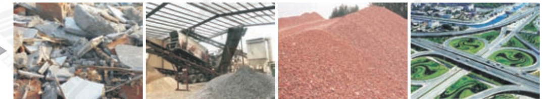
回收废料 recycling waste 破碎、筛分 crushing and screening 再生骨料 recycled aggregate 城市建设 urban construction
