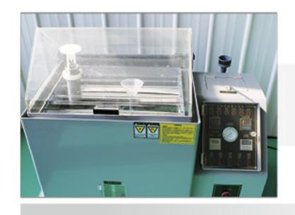
Salt spray tester: test the corrosion resistance of coating ( galvanized )
