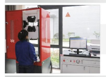
Hydraulic universal testing machine: test the mechanical properties: tensile strength, yield strength, elongation
