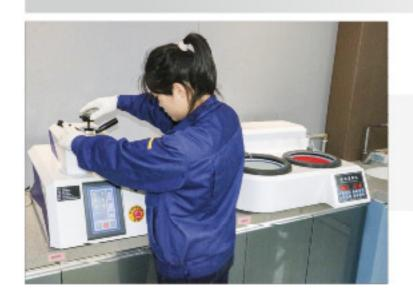
Metallographic analyzer: used to identify and analyze the structure of various metals and alloy materials
