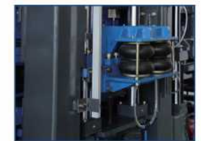
压头位移装置 Mould Head Shifting Device
