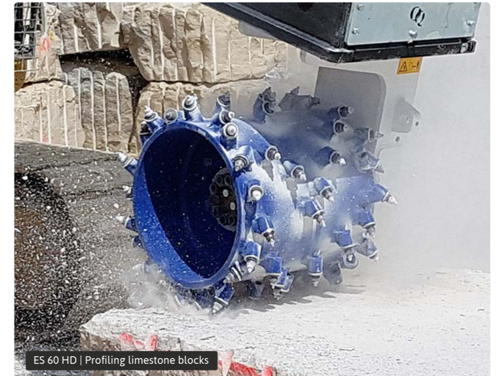
ES 60 HD | Profiling excavation boundaries
