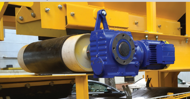
Shaft-mounted inverter-controlled motor
