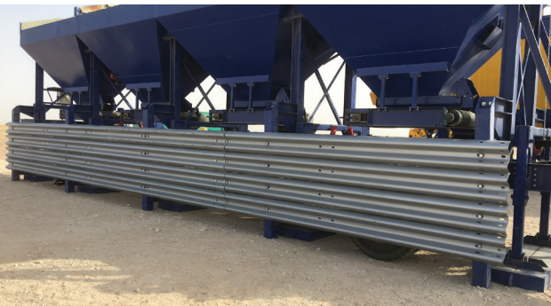
Built-in retaining wall
