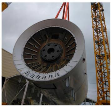
One of the biggest microtunnelling's technique's advantages is the possibility, within a certain diameter range, to easily increase the machine boring diameter by simply installing a removable "Upsizing Kit" which is easily bolted onto the original machine can.
