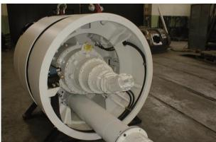
A cutterhead is attached to the machine; this is conceived and accurately designed both according to the specific geology of the ground to be excavated and to the main machine specifications in such a way to obtain the best possible advance rates with minimal cutting tools replacements.
