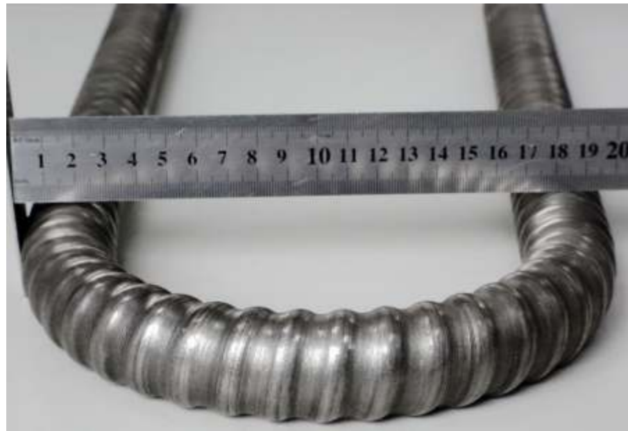
180 U-shape | No visible crack | No break
