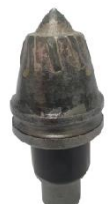
Model:3060-N9 Alloy size: 22 / 28 The steel body is thickened with 3060 steel body with 9 alloy bars. Suitable for cobblestone, sandstone, red sandstone and other hard rocks. Especially suitable for medium hard rock strata where steel body wear too fast.
