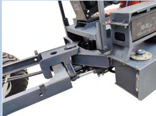
ARTICULATED STEERING STRUCTURE
