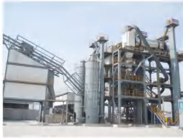
AMP4000-PRD2000沥青热再生搅拌站江苏兴化 AMP4000-PRD2000 asphalt hot recycle mixing plant used in Xinghua, Jiangsu Province
