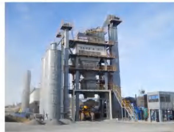
AMP4000型沥青搅拌站山东青岛 AMP4000 model asphalt mixing plant used in Qiangdao, Shandong Province
