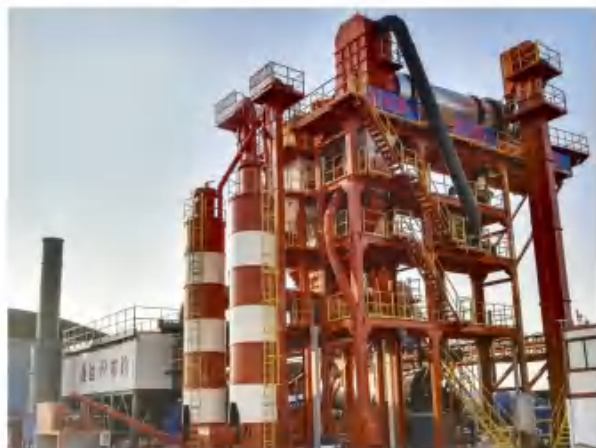
AMP2000-PRD1000沥青热再生搅拌站山东莱州 AMP2000-PRD1000 asphalt hot recycle mixing plant used in Laizhou, Shandong Province
