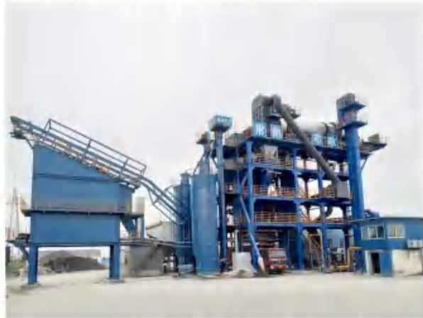
AMP3000-PRD1500沥青热再生搅拌站江苏苏州 AMP3000-PRD1500 asphalt hot recycle mixing plant used in Suzhou, Jiangsu Province
