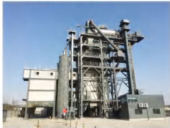
AMP3000-PRD1500沥青热再生搅拌站江苏无锡 AMP3000-PRD1500 asphalt hot recycle mixing plant used in Wuxi, Jiangsu Province
