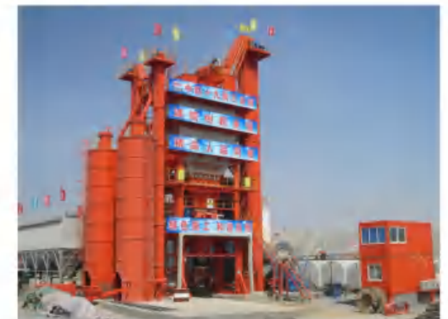
中铁十九局三处购买的AMP5000型搅拌站用于辽宁皮炮旺南高速 AMP5000 model asphalt mixing plant used in Liaoning Pipo-Wangnan expressway
