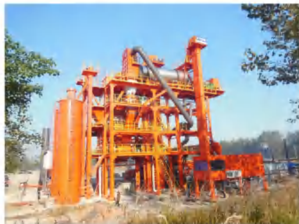
AMP3000-PRD1000沥青热再生搅拌站江苏淮安 AMP3000-PRD1000 asphalt hot recycle mixing plant used in Huai'an, Jiangsu Province
