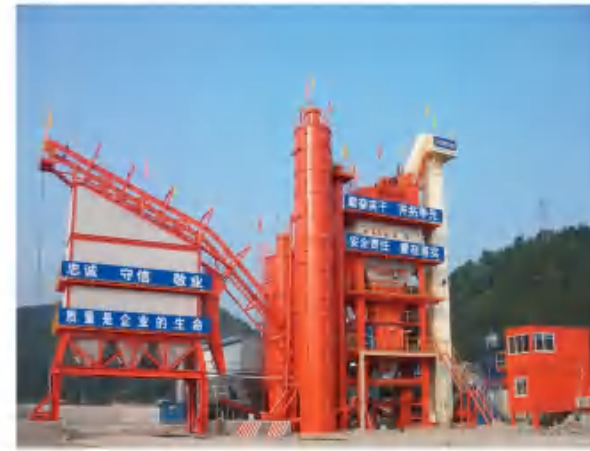
中铁十四局购买的AMP5000型搅拌站用于福建福泉高速 AMP5000 model asphalt mixing plant used in Fujian-Fuquan expressway
