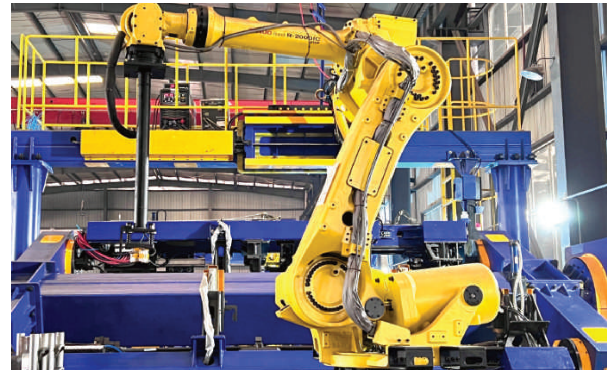
Fishplate Intelligent Welding Robot
