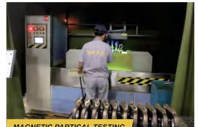
MAGNETIC PARTICAL TESTING
