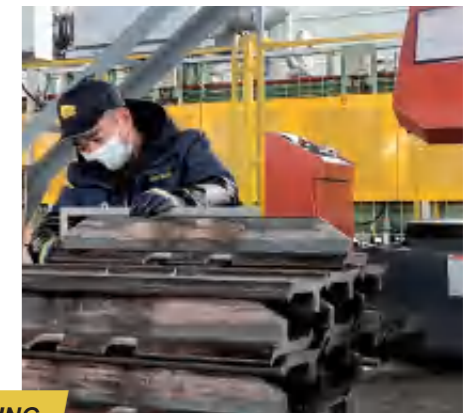
MAGNETIC PARTICAL TESTING
