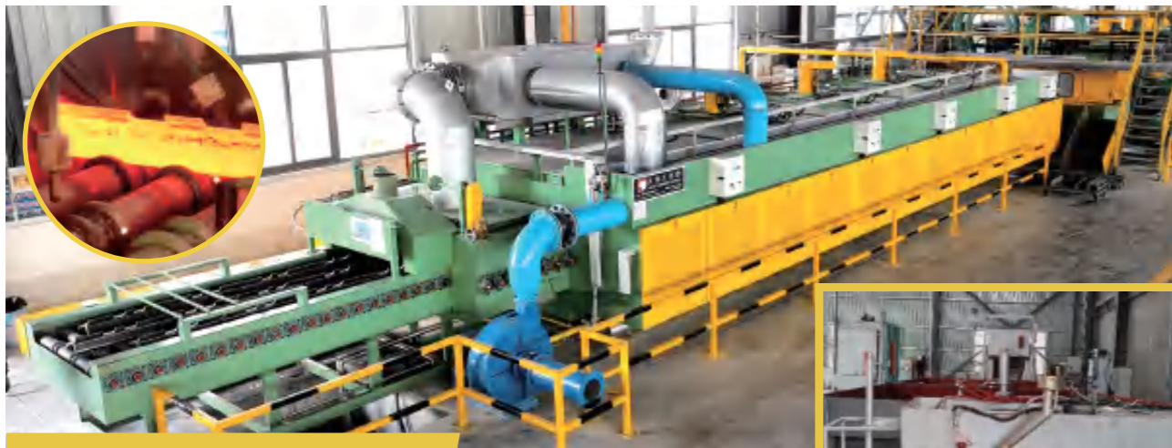
CONTINUOUS HEAT TREATMENT LINE
