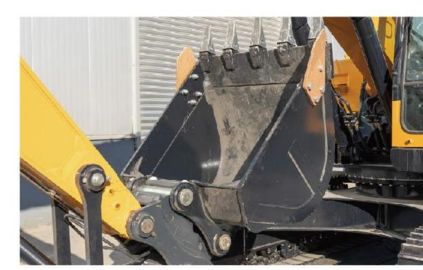
Made from high-strength wear-resistant steel, its cutting edges are hardened for enhanced durability, effectively resisting wear from sandstone, soil, and various materials.
