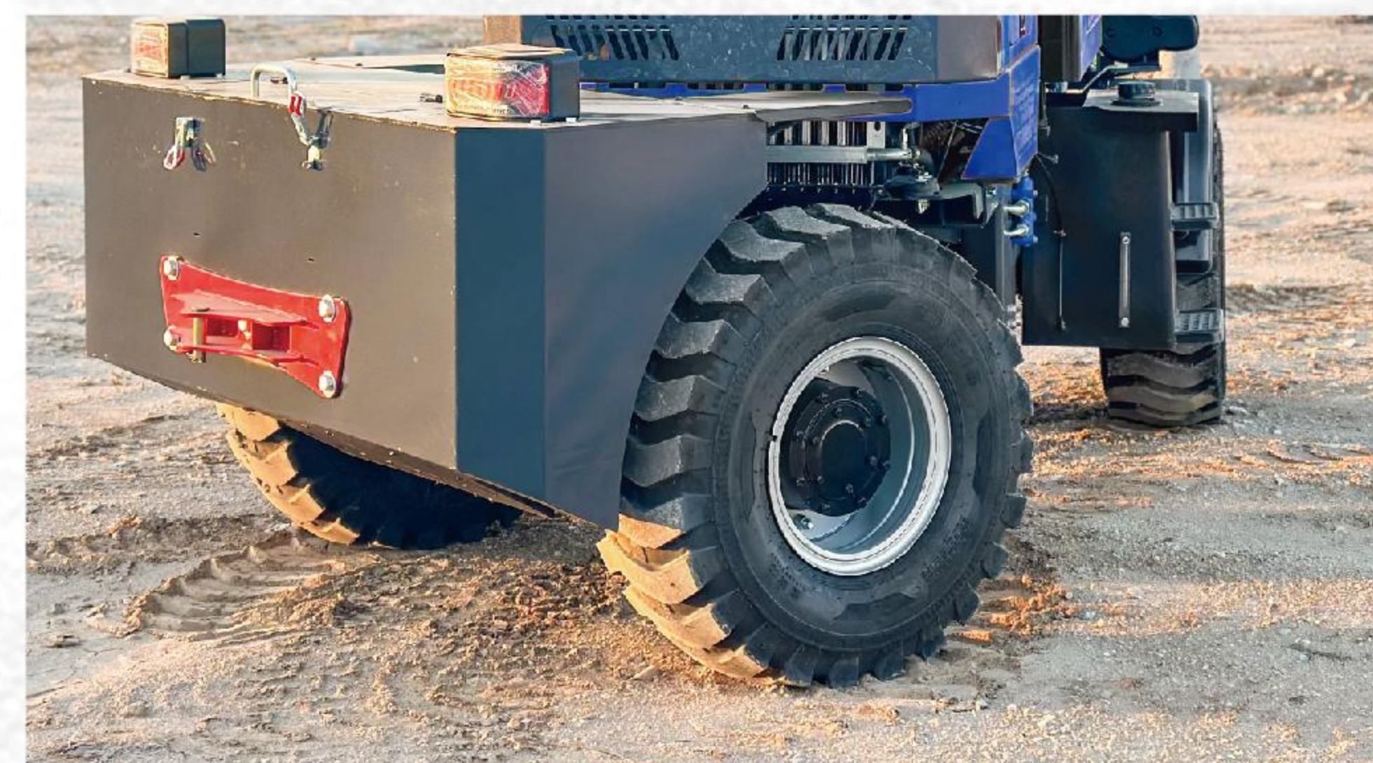
Rear wheel steering for heavy loads without tilting in turns, strong off-road performance.
