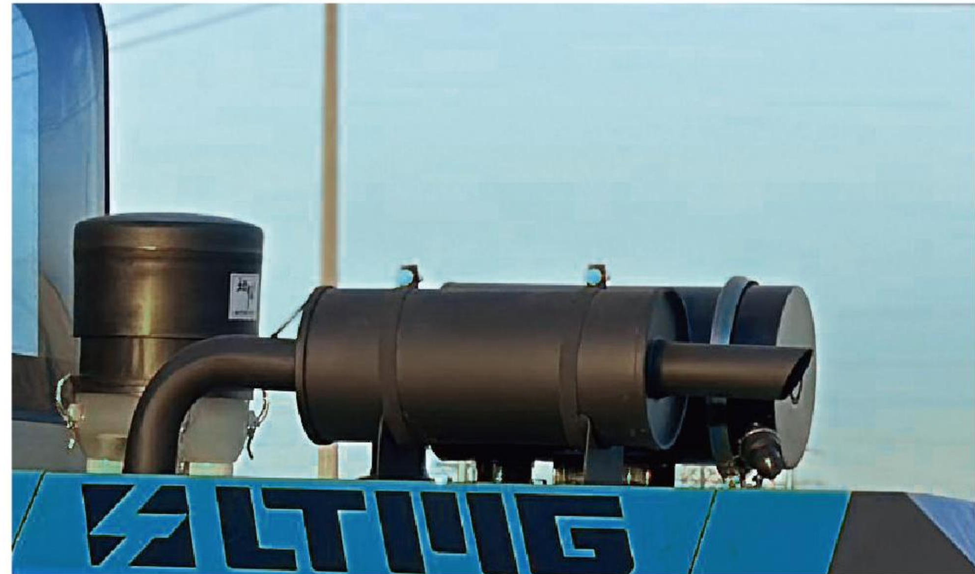
High-quality air filters to meet different emissions, realize the second muffling of the engine and reduce exhaust resistance at the same time.
