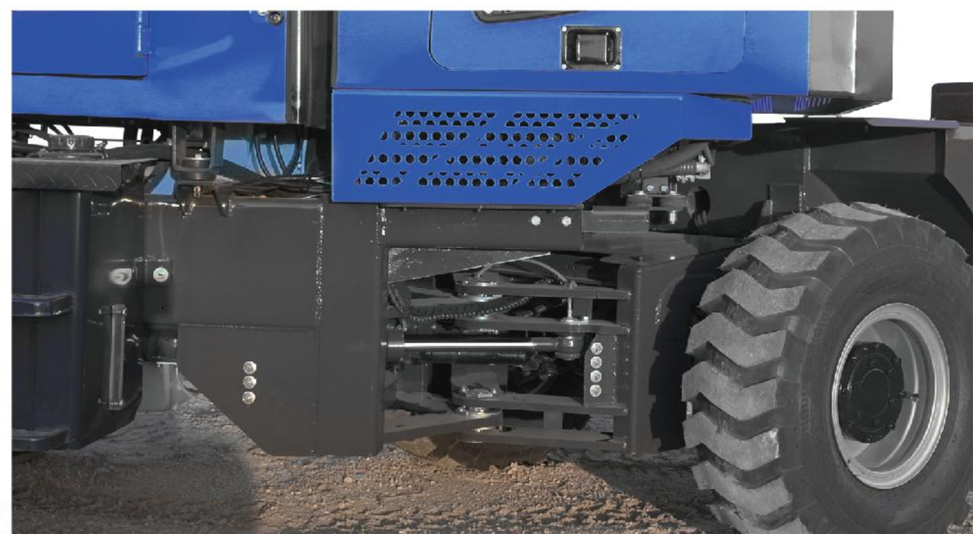
The articulation point is located in the rear design, small turning radius, stable center of gravity, not easy to rollover
