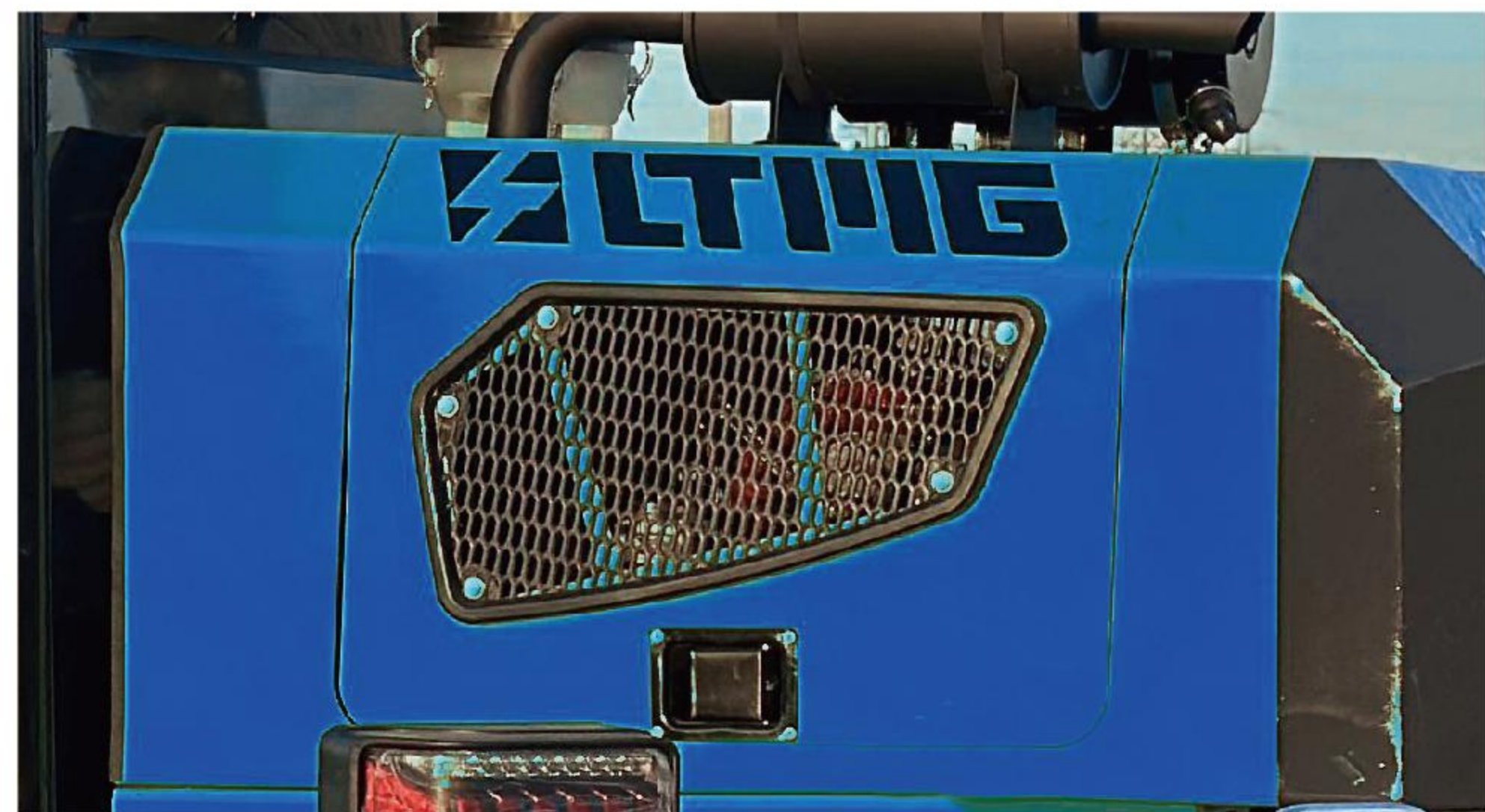
Honeycomb cover design, good heat dissipation performance, easy to access and maintenance.
