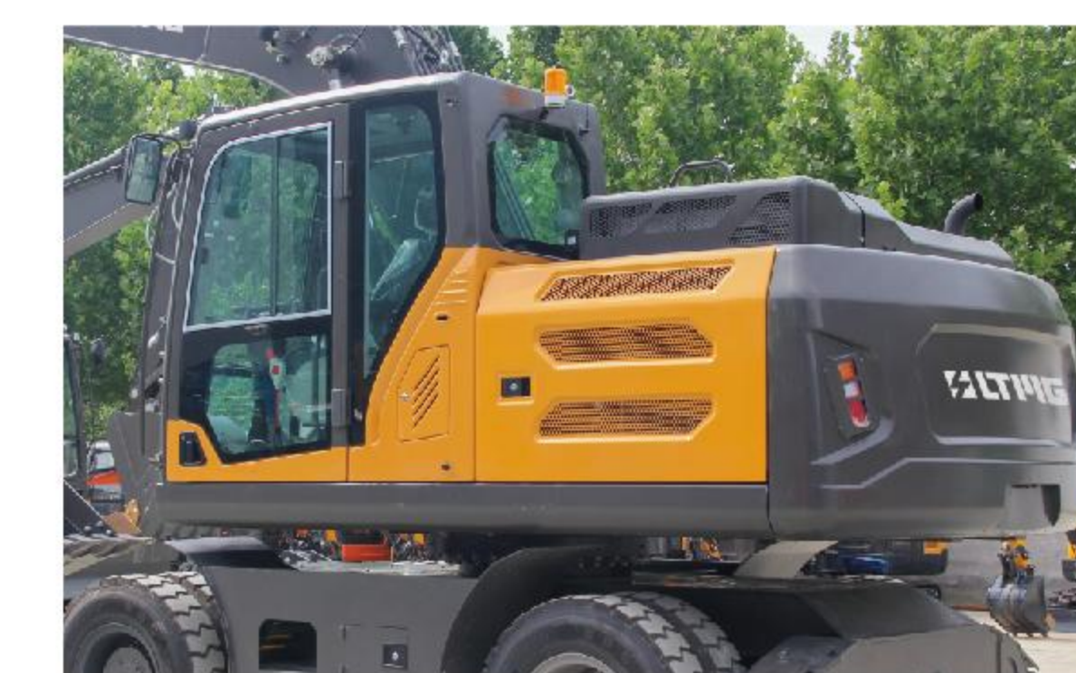
Upper platform cladding with low profile design for better side visibility for the driver. 上平台覆盖件采用低身位设计, 使驾驶员拥有更佳的侧方位视野。
