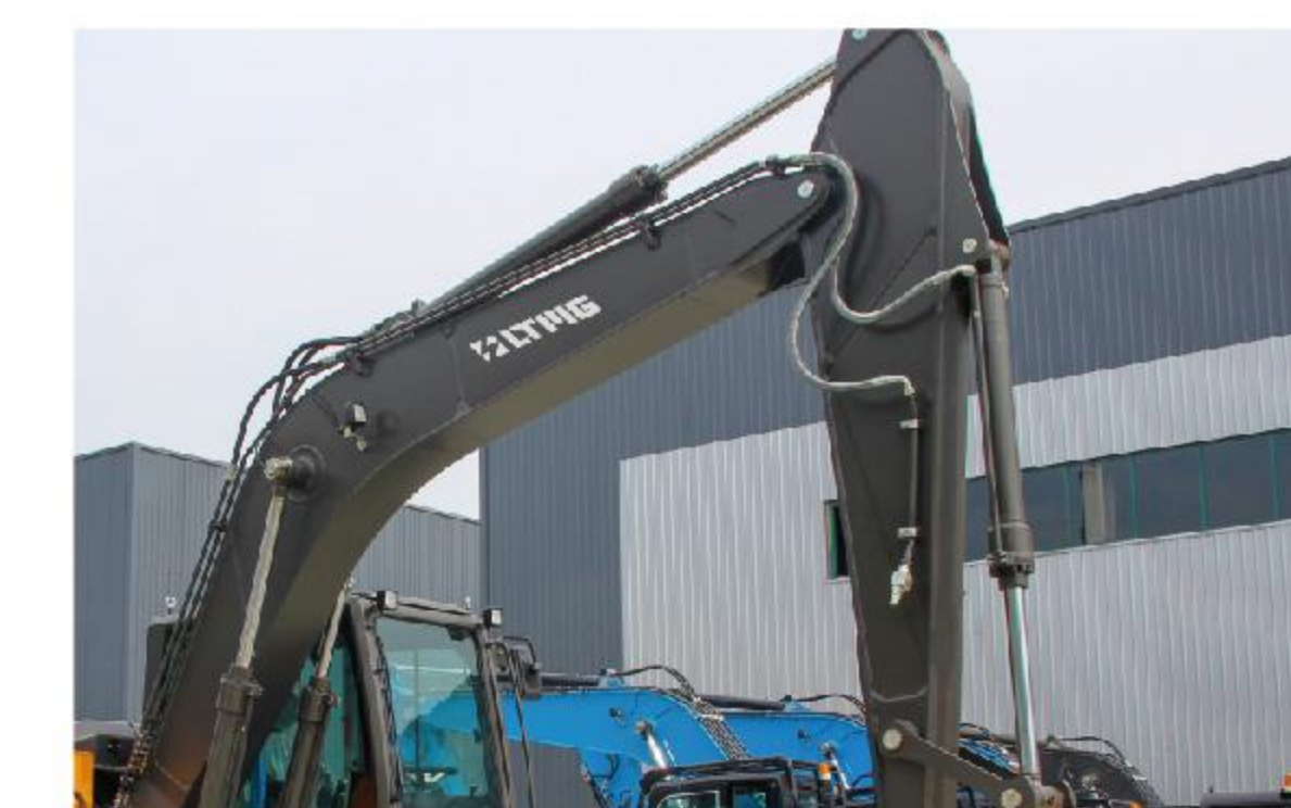
The boom adopts closed box type welded structure, strengthened main boom support, good overall torsion resistance. 动臂斗杆采用封闭箱体式焊接结构, 强化型主臂支撑, 整体抗扭性能好。
