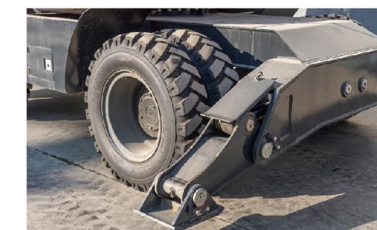
Outrigger design for safe and stable operation. 支腿设计, 作业安全稳定。
