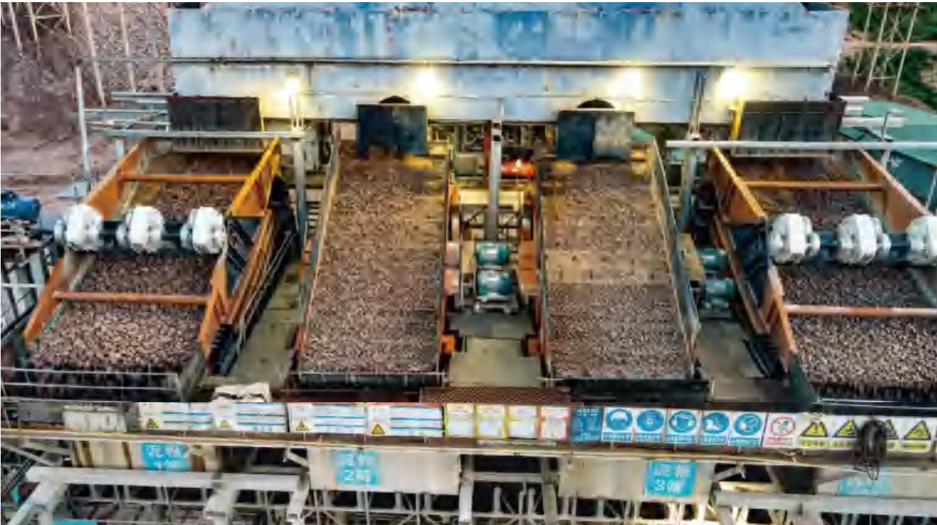
直线主动行进, 筛分精度高;多组厢式激振器提供足够激振力;科学分析根据工况定制;延用德国工艺, 运行正常稳定可靠;提供特有隔振架, 启停平稳, 对基础的动载荷减少99% Linear active travel, high screening accuracy; Multi-group chamber exciter provides sufficient excitation force; Scientific analysis is customized according to working conditions; Continued use of German technology, stable and reliable operation; Provide unique vibration isolation frame smooth start and stop, reduce the dynamic load on the foundation by 99%
