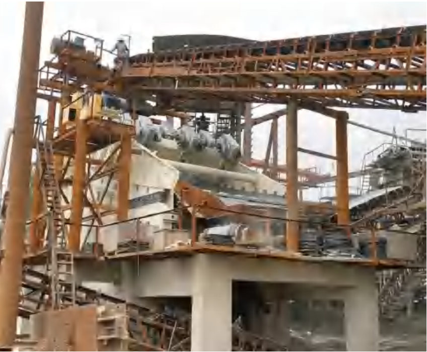
筛机起机和停机过程平稳，对基础无共振 Screen machine start and stop process is stable, no resonance to the foundation
