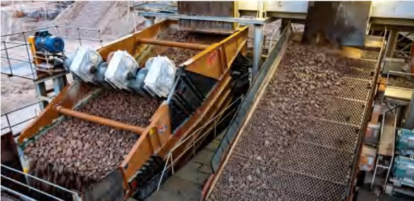
筛机的高频振动加上橡胶筛网的二次回弹, 避免了筛网堵孔现象 The high frequency vibration combined with the secondary rebound of the screen avoids the hole blocking of the screen
