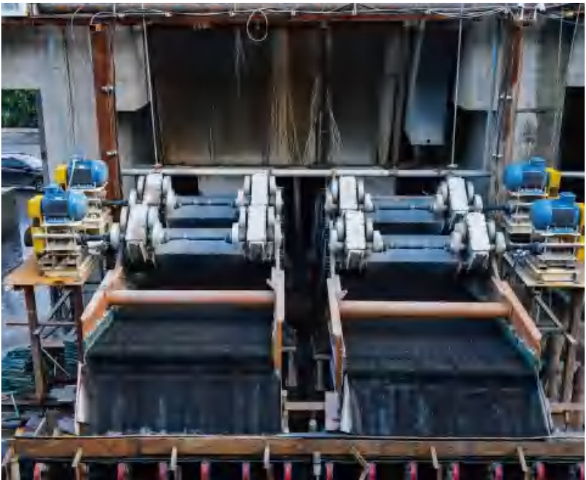
采用了隔振架装置,启停机非常平稳,使土建基础更安全。 Using the damper frame device, start and stop very smooth, make the civil foundation more secure.
