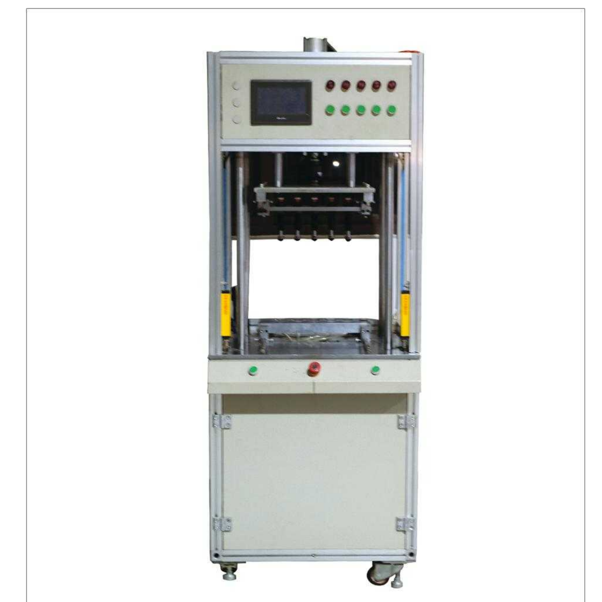
Level Gauge - Air Tightness Testing Platform
