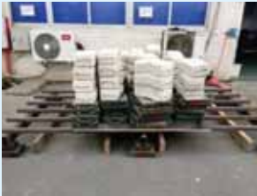
Loading Capacity Test
