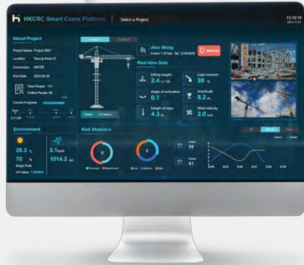
CMP (Central Management Platform)
