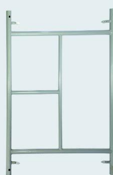
RFH-C007A 门架 Frame 1360x1000mm Dia 48.3x2.65mm
