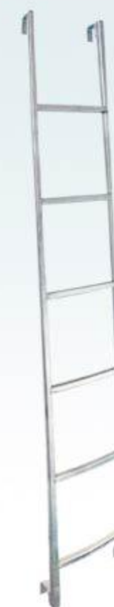
RFH-G022D 梯子 Ladder 2220x300mm/6.79kg 40x20x2mm 20x20x2mm
