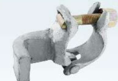
RFH-A056 焊L板扣件 Single Coupler with Welded L-Plank 48.3mm 0.84kg
