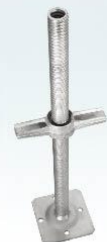
RFH-B011A 空心调节底座 Hollow Screw Jack Base 600,914,1524 mm Φ 32/35/38x4mm 143x143x5/6mm
