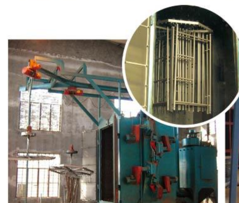
喷砂处理设备 Sandblasting treatment equipment
