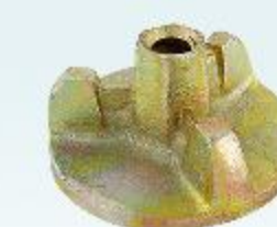
RFH-FW009K 加强型夹器螺母 Reinforced Type Anchor Nut 0.8Kg/Dia110mm 1.2Kg/Dia130mm Φ 17
