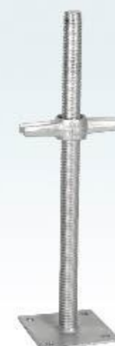
RFH-B011A 空心调节底座 Hollow Screw Jack Base 600,914,1524 mm Φ 32/35/38x4mm 143x143x5/6mm
