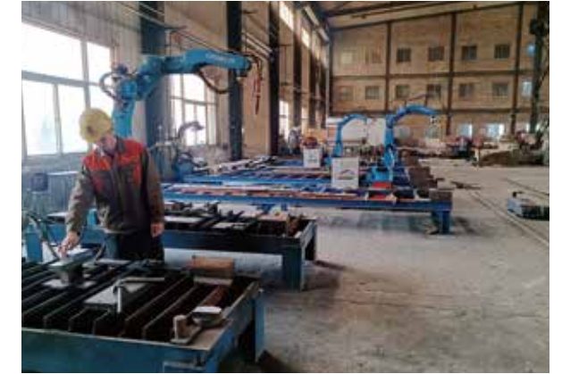
下料火焰切割 Blanking flame cutting
