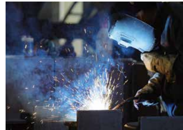
气体保护焊接 Gas shielded welding
