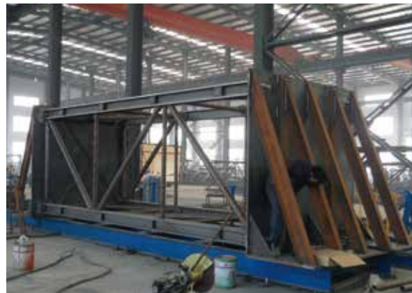
部件工装卡具 Component tooling fixture
