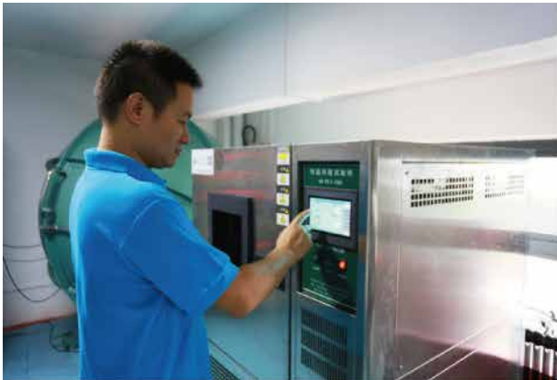
High-Low Temperature Test machine 高低温环境试验箱
