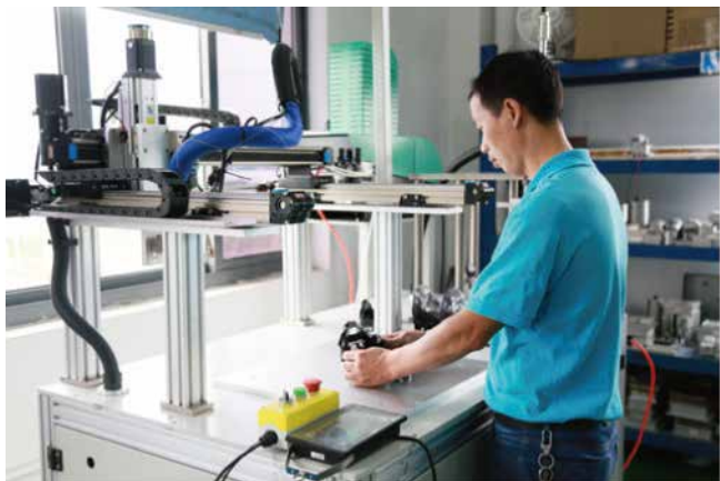
Hot Melt Glue Automatic Three-axis Platform 热熔胶自动三轴平台
