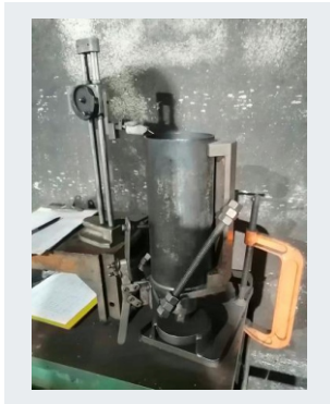
▲ Inspection of verticality of the inner tube
