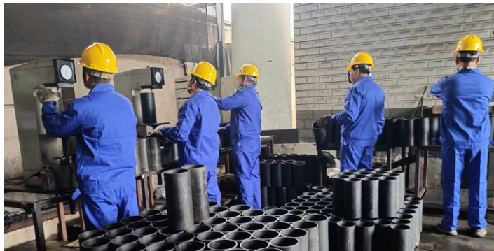
▲ Quenching of the inner tube – temperature in the quenching furnace is 860 \pm 10^{\circ}\text{C} , oil temperature is 45\text{--}70^{\circ}\text{C} , and the time is 210 seconds.
