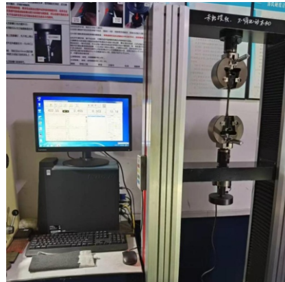
▲ Tensile machinery performance testing of the outer tube
