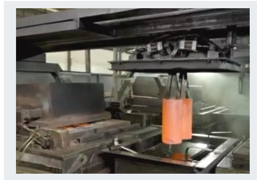
▲ Quenching of the inner tube – temperature in the quenching furnace is 860 \pm 10^{\circ}\text{C} , oil temperature is 45\text{--}70^{\circ}\text{C} , and the time is 210 seconds.
