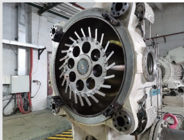
刀盘拆解 Dismantle Cutterhead
