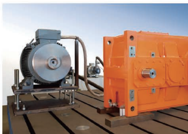
125KW带封闭循环冷却的试验平台 125KW Test Platform with Closed Circular Cooling System
