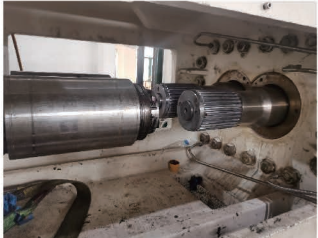
螺杆回装、调相位 Reinstall the Screw and Adjust Phase
